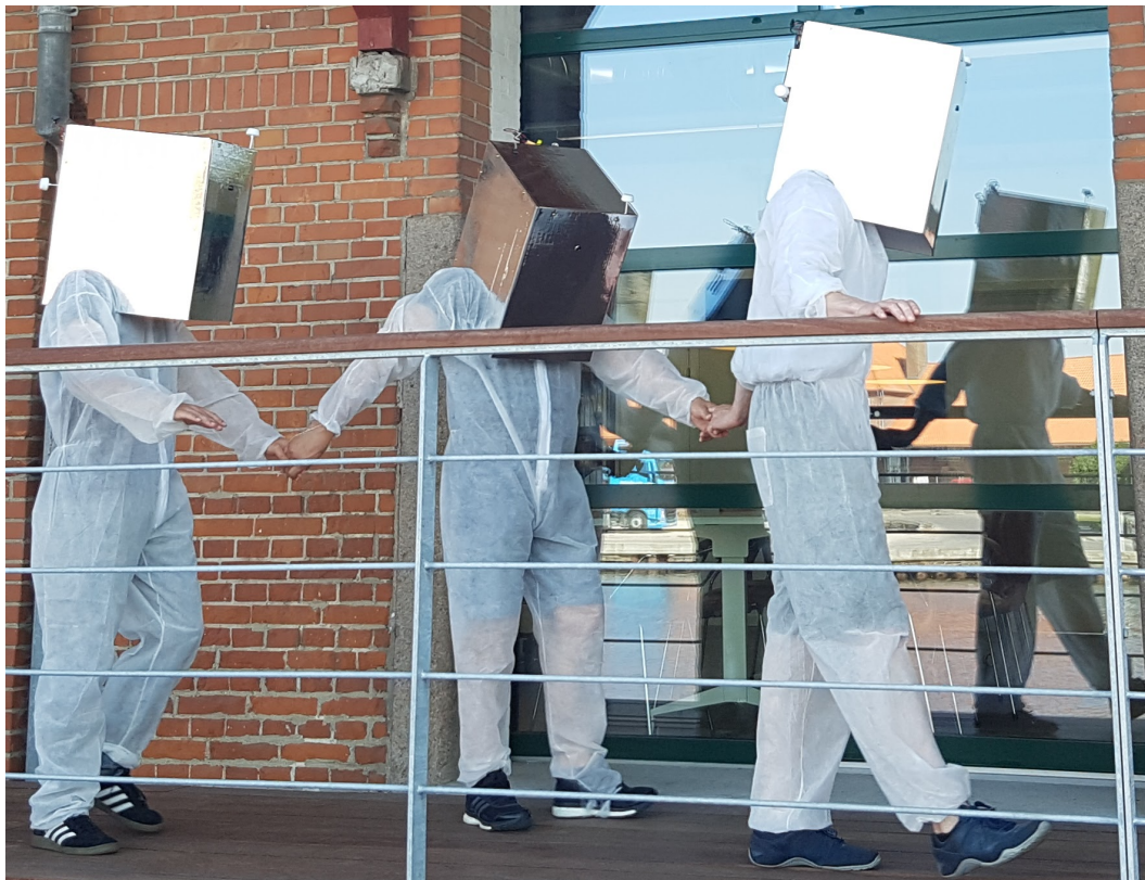
Figure 1. Three headset wearers attempt to explore the world together. A screen inside each helmet is receiving a visual stream from a camera mounted on the front of another wearer’s helmet. An Arduino rapidly and automatically switches the camera transmissions between different headsets.
