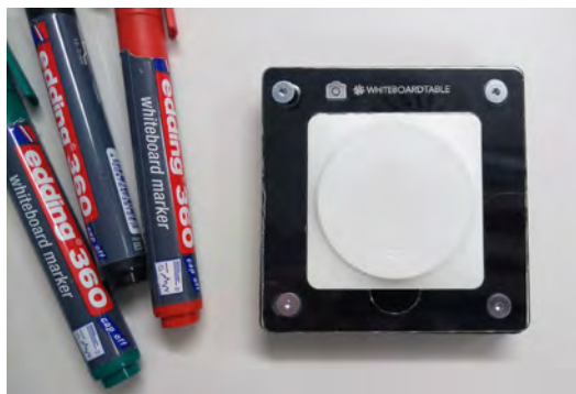
Figure 4. The cameras above the whiteboard table are triggered by this white Logitech POP button, which was placed in a black, laser-cut casing (whiteboard markers for scale).
